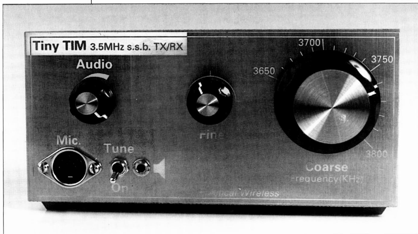
The Completed PW prototype Tiny TIM (Transceiver In Miniature) 3.5MHz s.s.b. project, designed by Tim Walford G3PCJ.
