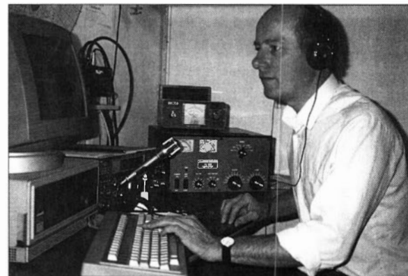
Fig. 2: The 'final' power for the AL-80BX unit is provided by a 3-500Z valve, with a warm-up time of 10 seconds.
